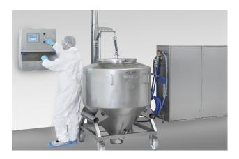
All of the components for transporting and treating the cleaning water are stored within a compact stainless steel cabinet. Washing processes are performed on the basis of recipes and are automatically logged. A touch panel on the device enables convenient local operation.
